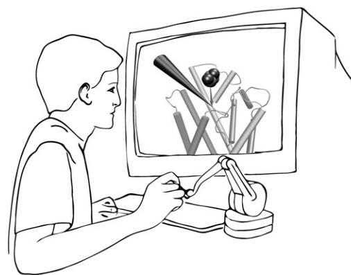
FIGURE 1 Our system for IMD. A customizable view of a running simulation is displayed on a desktop PC as it is computed. The PC displays a pointer that corresponds to the position of the haptic device used to interact with the system. A researcher uses this haptic device to apply a downward force to a simulated molecule of glycerol, feeling resistance in his hand as it moves through the channel.
